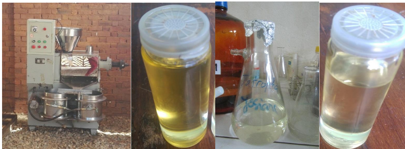
Figure 2. Semi-industrial oil press
